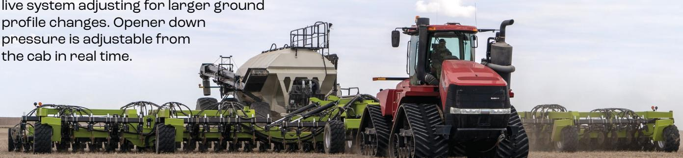
Outfitted with our exclusive 8621 Gent undercut disc openers – the easy-to-pull Spyder Drill provides ultra-low soil disturbance, virtually no hairpinning and lower fuel consumption.
